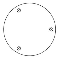
2. Drill three holes according to the supplied **Template Plate**, and insert the supplied **Plastic Anchors** into the holes.
