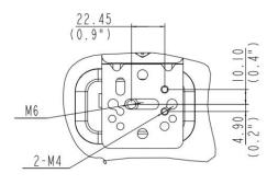
Detail A There are two threaded hole bosses installed in the project.
