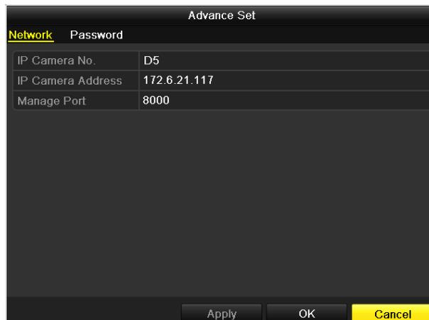
Figure 2. 15 Network Configuration of the Camera
