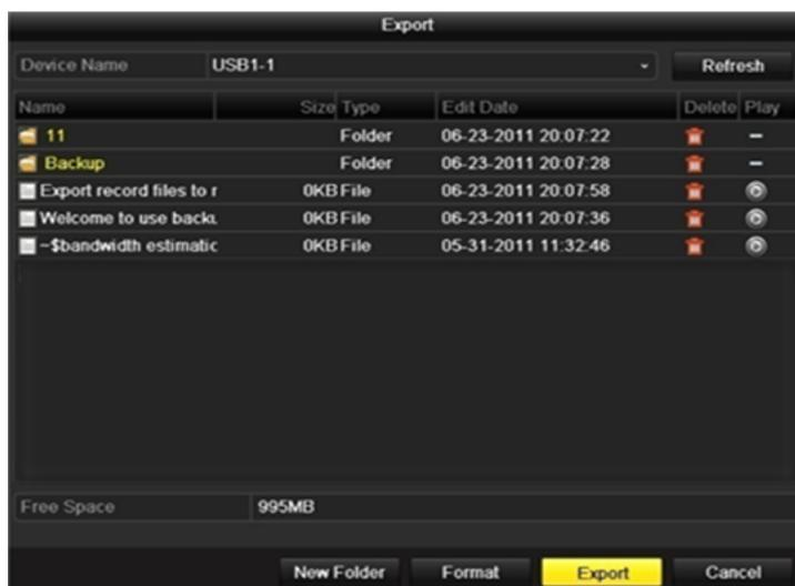
Figure 7.27 Export Video Clips Using USB Flash Drive
