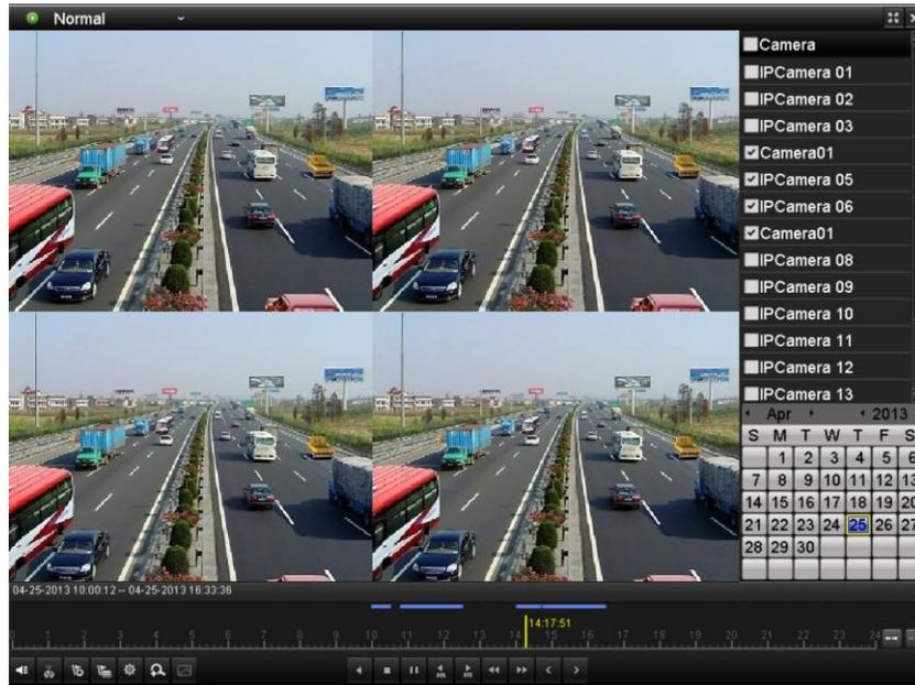
Figure 6. 27 4-ch Synchronous Playback Interface
