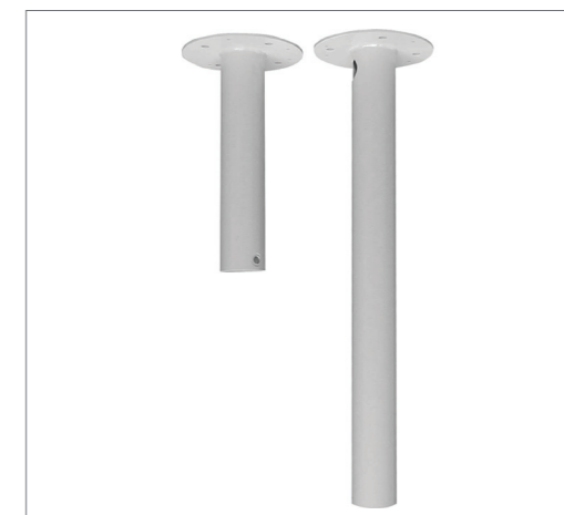
Straight Tube Height: 250/500 mm (9.8/19.7 inches) ,Diameter: 50 mm (2 inches) 1 kg (2.2 lbs) / 1.8 kg (4 lbs), Supplied with rubber washer-8x1, Pendant tube washer-1, spring washer-8x1 and waterproof rubber-1, M8*12 screw-1.
