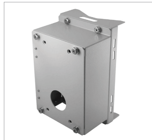
POLE WIDE BOX MOUNTING 270x166x155 mm (10.6x6.5x6.1 inches); 3.2 kg (7.1 lbs); Supplied with M8*16 screw-4, washer-4, spring washer-4, stainless steel straps-4.
