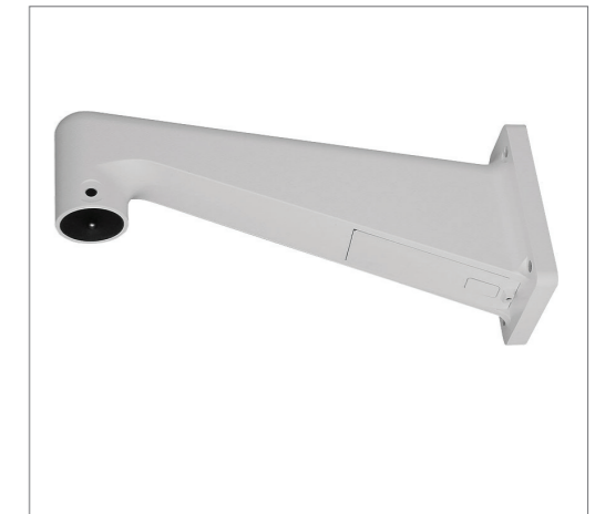
Standard Pendant Mount 348x104x138.6 mm (13.7x4.1x5.5 inches); 1.5 kg (3.3 lbs); Diameter: 45 mm (1.8 inches). Supplied with rubber washer-8x1, Pendant tube washer-1, spring washer-8-1 and M8*12 screw-1.
