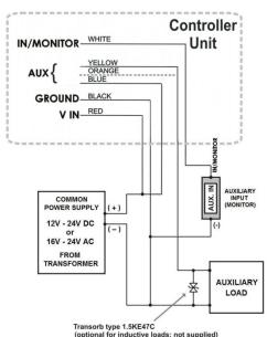
Figure 5: Pre-Wired Connection for Auxiliary Input & Output
