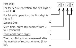
For example **0 5 1 2** means: fail secure operation (0), with5 minutes Siren time (5) and a 12-second Lock Strike Release time (12).
