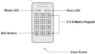
Figure 2: AC-S43 Front Panel
