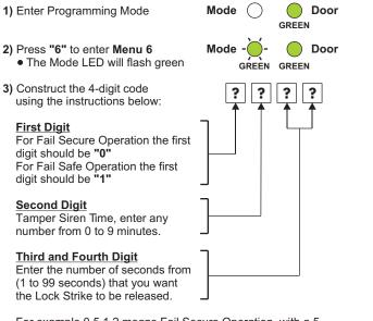
For example 0 5 1 2 means Fail Secure Operation, with a 5 minute Tamper Siren Time, and a 12 second Lock Strike release time.
