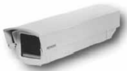
CHH Camera housing 320 mm, IP66, quick connector, 230 V heater
