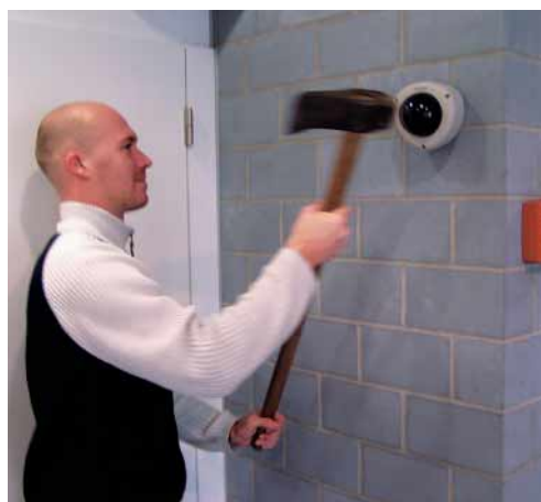
1000 kg impact resistant and IP66 protection rating
