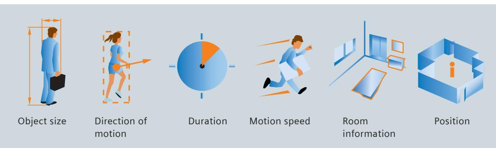
Eyetec™ is the first motion detector with comprehensive information on movements and room conditions.
