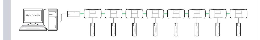
A maximum of eight doors can be programmed from a PC using SiPass Entro Lite software and USB-RIF/2 reader interface.
