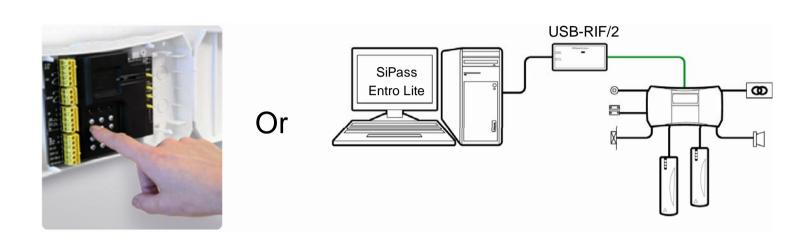
Programming inside the DC800 controller via the built-in keypad
