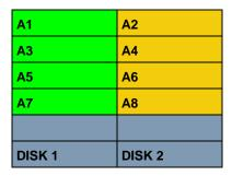
RAID 0 capacity is the size of the sum of the capacities of the disks in the RAID 0. For example, if you have four disks of sizes 1 TB, 2 TB, 3 TB and 2 TB respectively in one RAID 0 array, then the maximum capacity is 8 TB.
